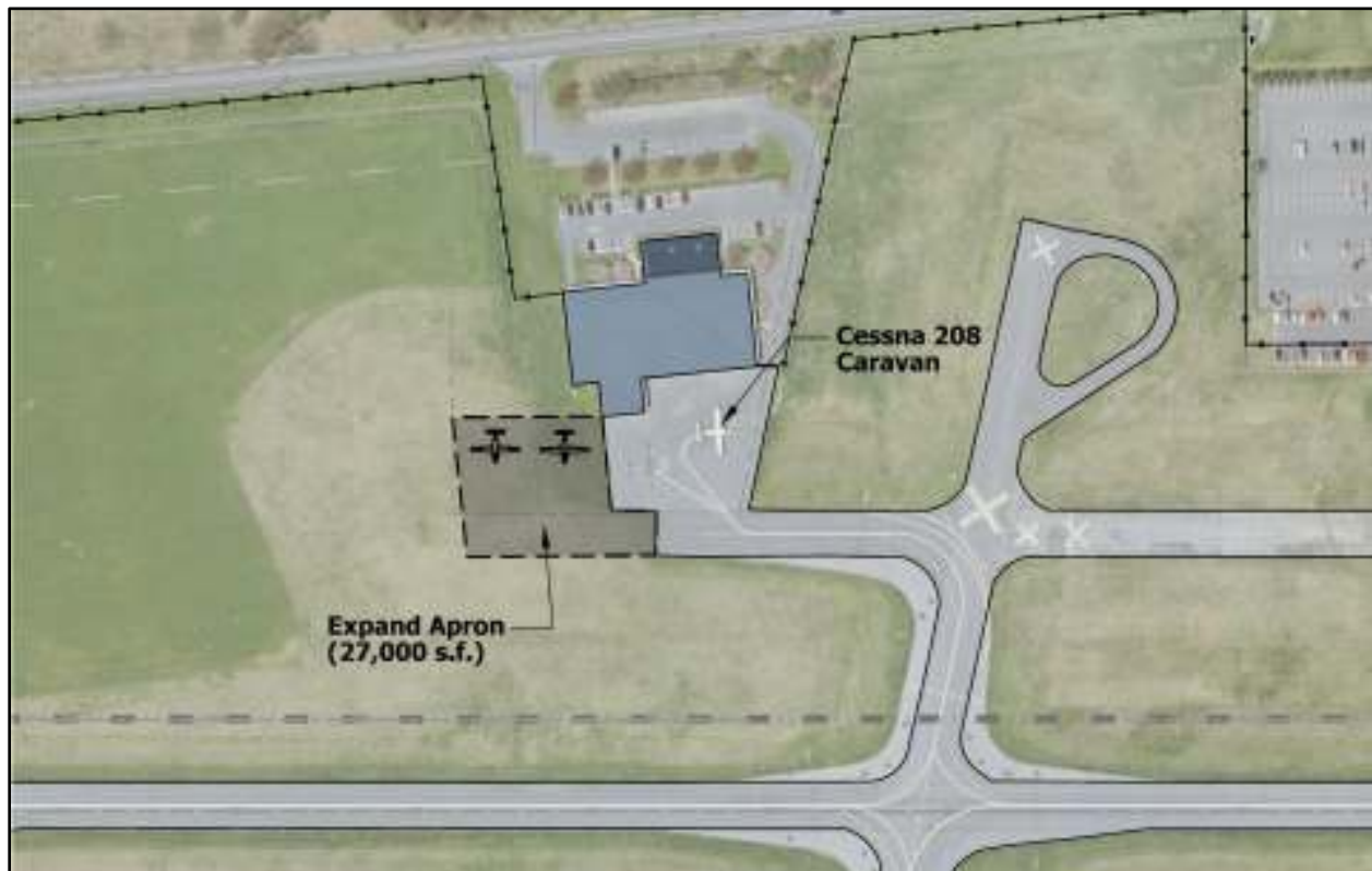
Figure 5-23: Alternative 14 – Air Cargo Apron Expansion
