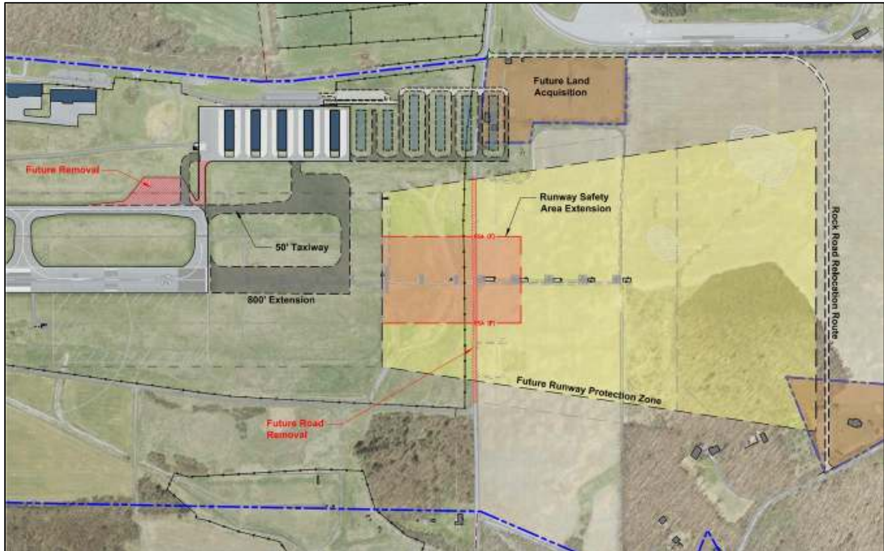
Figure 5-2: Alternative 2 – 800-Foot Extension at the Approach End of Runway 24
